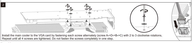
The thermal compound is already pre-applied to the heatsink. If the cooler has to be installed a second time, we highly recommend using the MX-4 from ARCTIC. Only this compound guarantees optimal performance in combination with the surface of our heatsinks.
